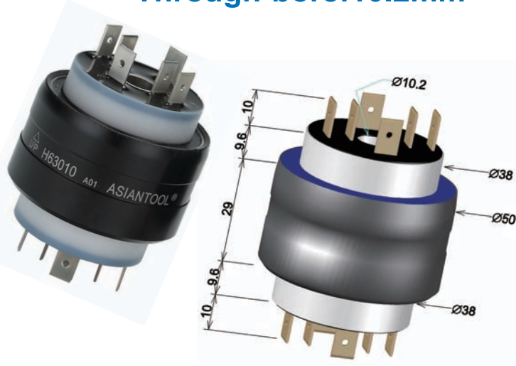
H63010 6poles/30A/AC250V Through-bore:10.2mm
