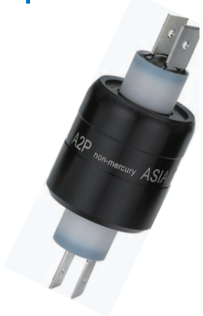
A2P NM (non-mercury) 2poles/30A/AC380V
