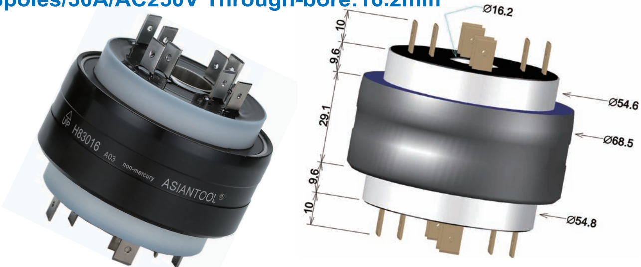
H83016 NM (non-mercury) 8poles/30A/AC250V Through-bore:16.2mm
